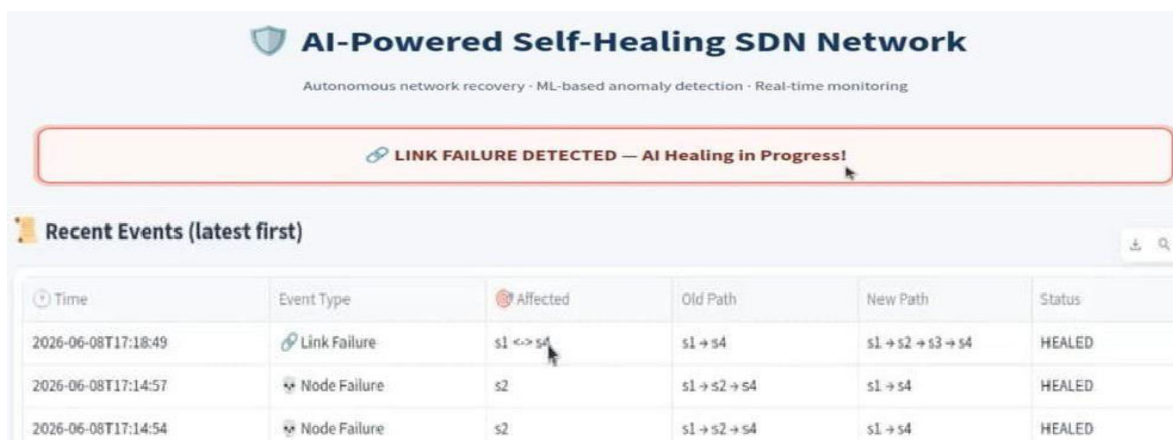
Fig.4. Link Failure Detection and Automatic Rerouting
